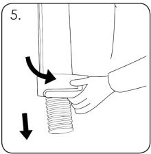
To remove the cups, move the quick release 45 degrees to the right.
